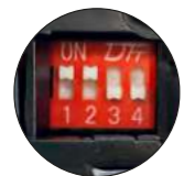
DIP-Switch power adjustment
